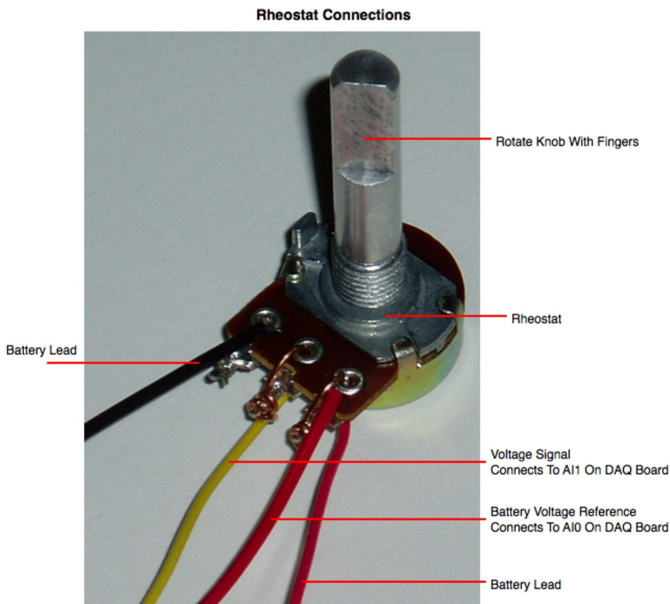
The following diagram shows how the rheostat is hooked to the DAQ device.
