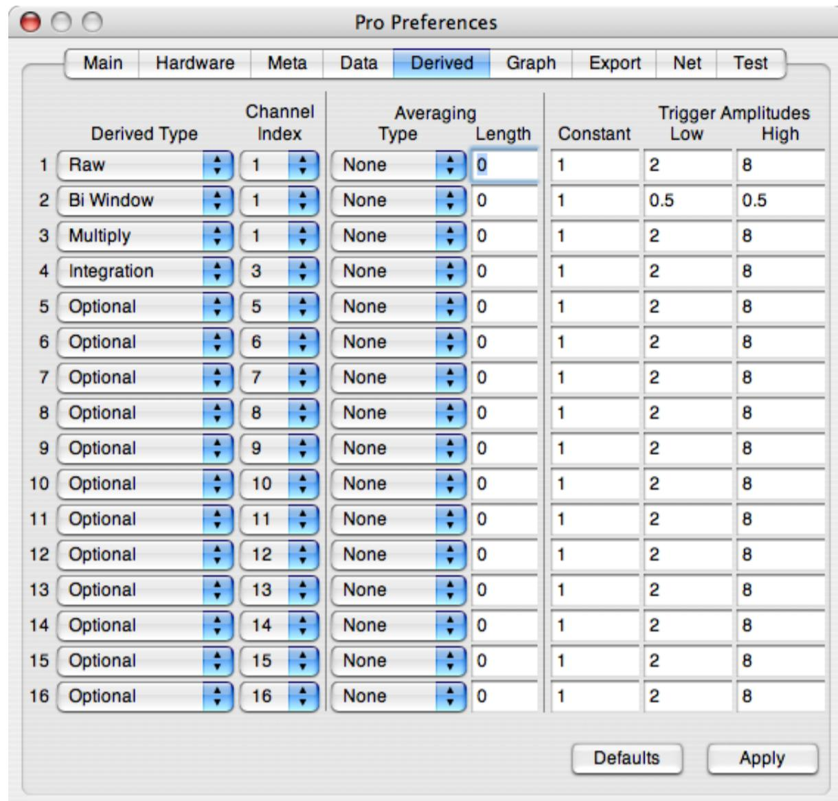
The mapping takes the voltage from channel 1, called the domain signal, and transforms it 4 times into the windowed integration, which is called the range signal.
