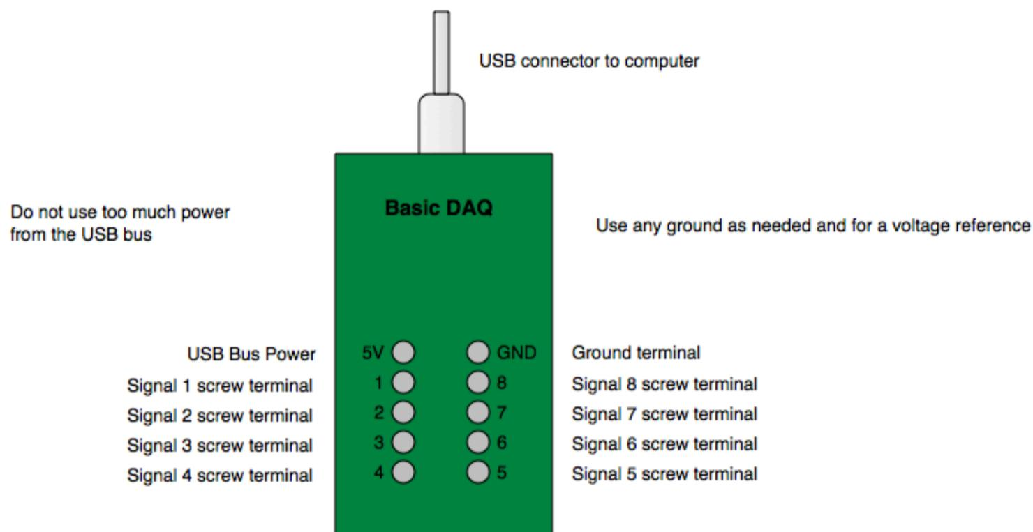
The screw connectors 1-8 correspond to the curve index in the signal window. Each connector is a single-ended connection to a digitizer. Typically, a sensor has a signal wire which can be attached to any of the signal connectors, usually in order one to eight for up to 8 sensors, a ground wire which is connected to the GND terminal and a power wire which can be connected to the USB Bus Power (5 V) connector. Make sure not to overload the power.
